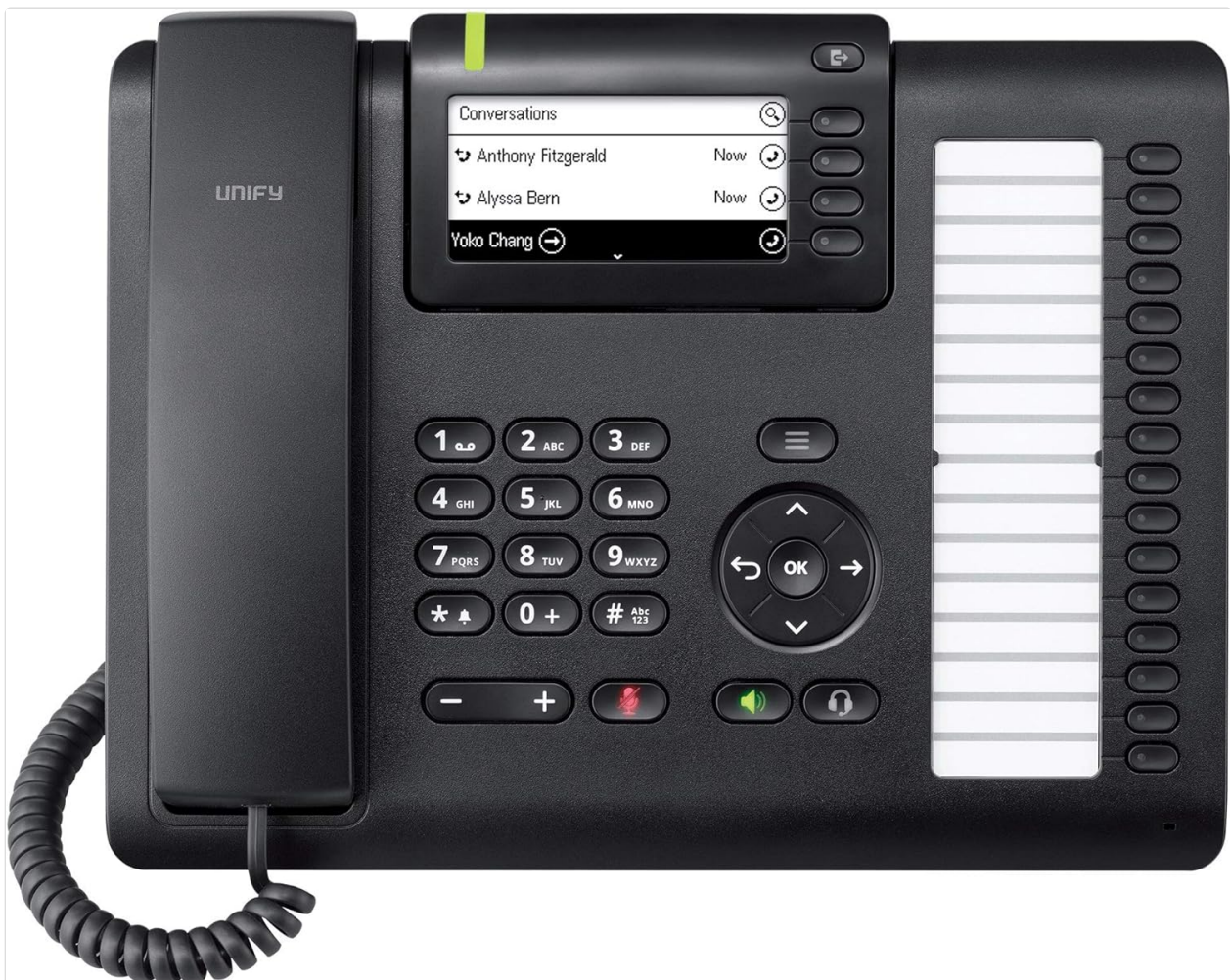
Figure 2.1: Angled view of the Unify Openscape CP400 Desktop Phone. This image shows the handset, main keypad, navigation cluster, display, and the array of programmable function keys on the right side.
