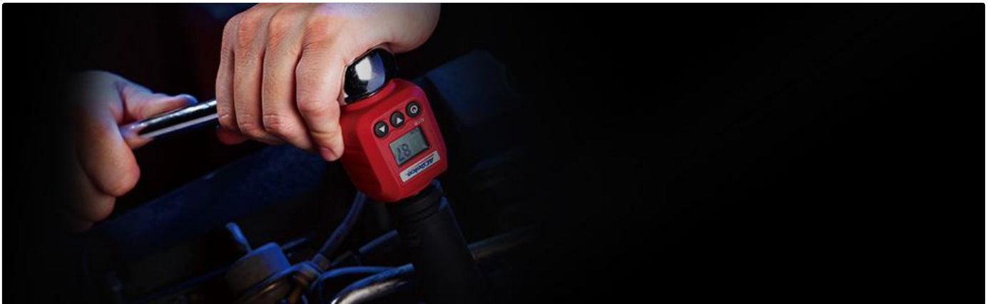
Image: The ARM302-4S in use, attached to a ratchet, applying torque to a component.
