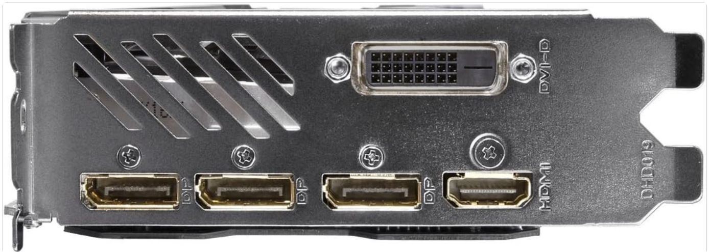
Image 5.1: Rear panel of the graphics card, featuring DisplayPort, HDMI, and DVI-D connectors.
