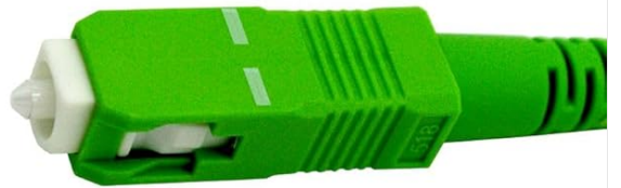
Figure 4.1: Always remove the dust cap and avoid touching the fiber end-face.
