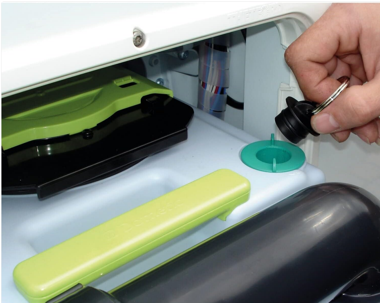
Figure 4.1: Illustrates the process of inserting the black sealing plug into the green cassette adapter, which is already integrated with the Dometic toilet cassette. This plug ensures a sealed system when the toilet is not in use or during transport.
