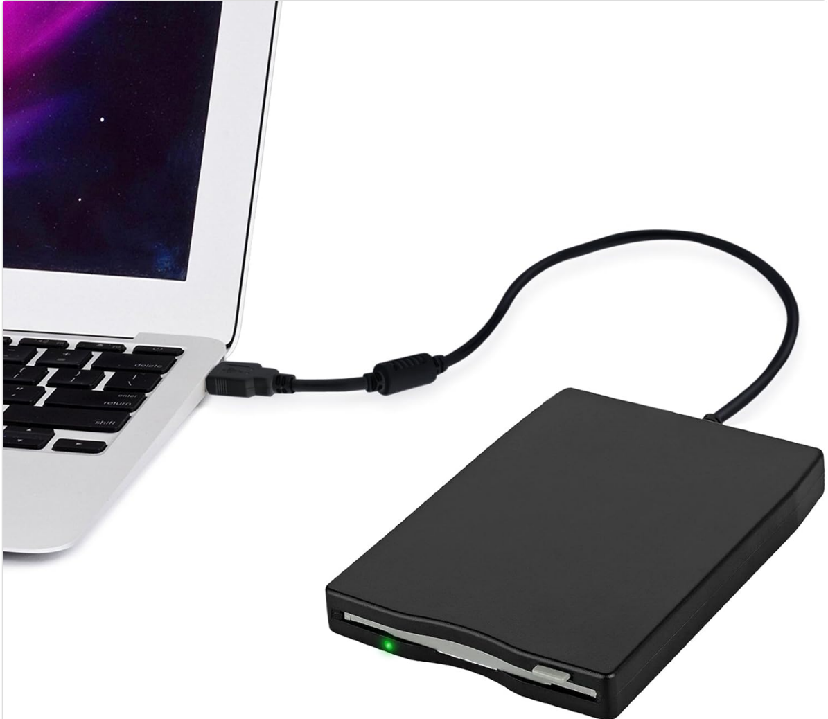
Image: The eSync USB Floppy Drive connected to a laptop, illustrating the USB-A connection.
