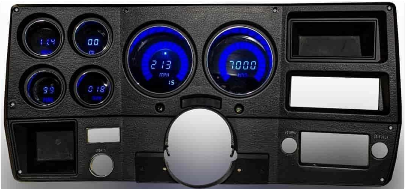
Figure 5.1: Fully assembled Intellitronix LED Digital Gauge Panel. This image shows the panel installed, displaying bright blue digital numbers for speed, RPM, fuel level, oil pressure, water temperature, and voltage.
