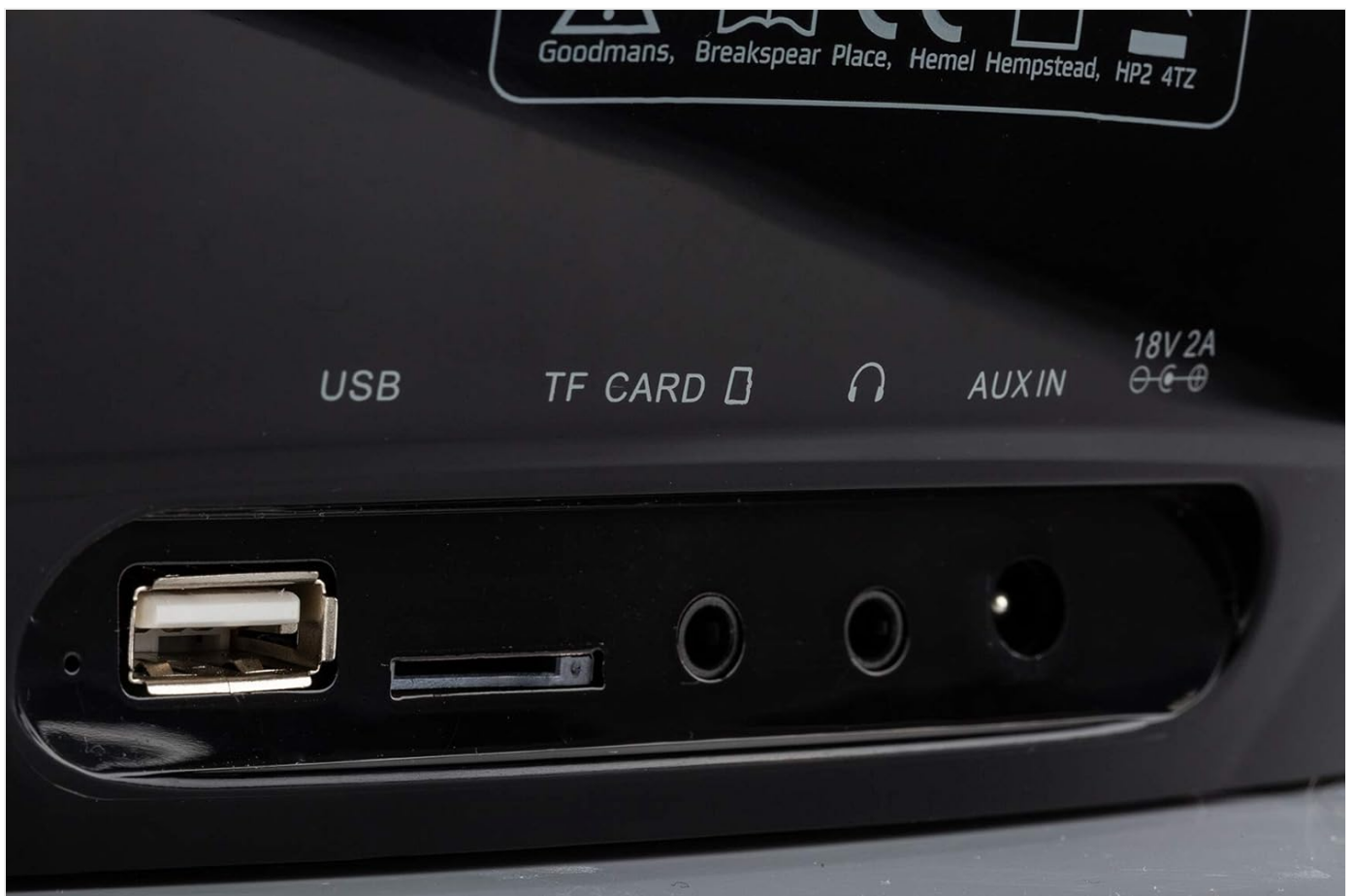
Figure 4: Close-up of the input ports located on the back of the speaker. From left to right, these include a USB port, a TF CARD slot, a headphone jack, an AUX IN port, and the 18V 2A power input.
