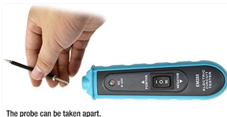
Image 3.2: The probe tip can be detached for maintenance or replacement.
