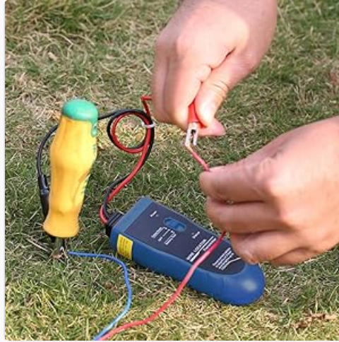
Figure 5.1: Connecting the Transmitter
