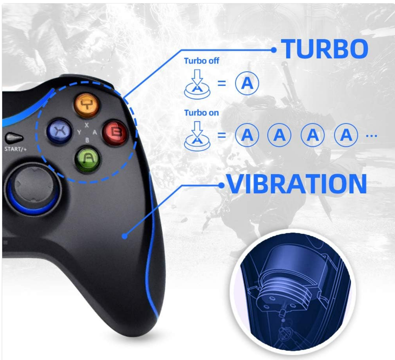
Image 4.1: Illustration of the Turbo function (repeated button presses) and the internal vibration motor for feedback.
