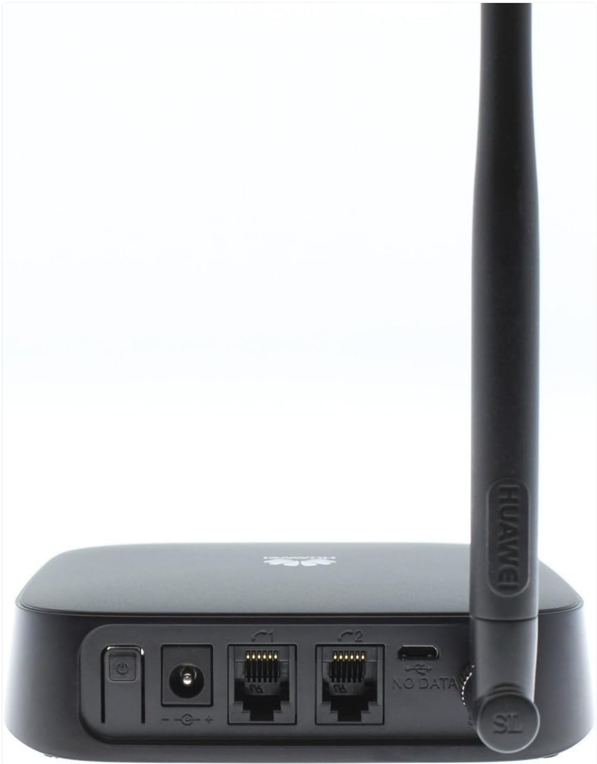
Figure 2: Rear ports of the Huawei ETS1162. This image displays the back panel of the device, highlighting the power input, two RJ11 telephone ports (labeled C1 and C2), a USB port (labeled NO DATA), and the antenna connection point.
