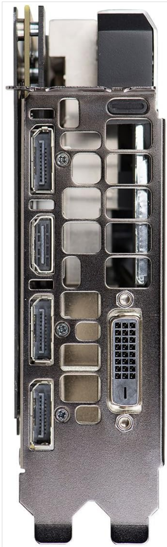
Figure 4: Display output ports on the EVGA GeForce GTX 1080, including DisplayPort, HDMI, and DVI.
