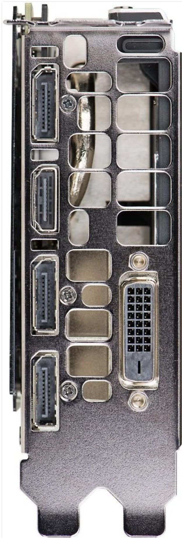
Image 4.2: Rear I/O ports (DVI, DisplayPort, HDMI).
