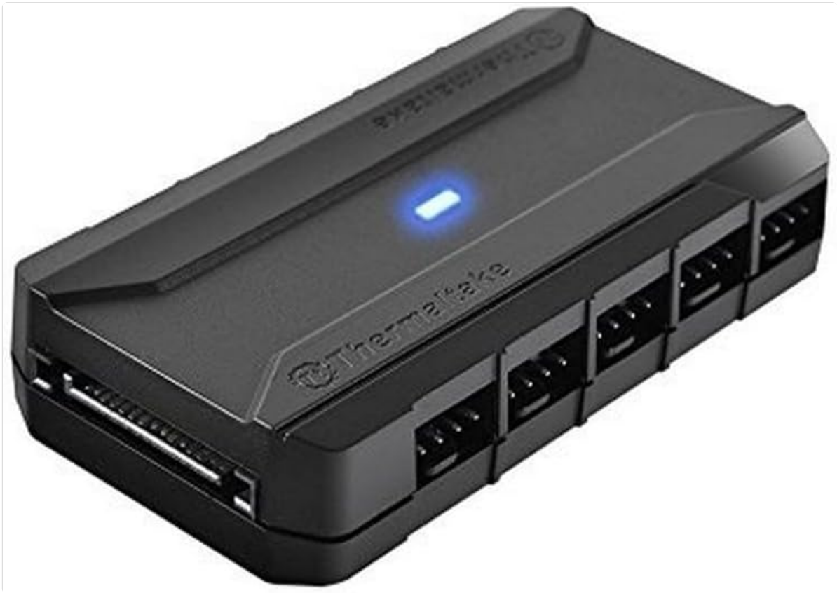
Figure 1: Front view of the Thermaltake Commander FP Fan Hub, showcasing its compact design and illuminated blue LED power indicator.
