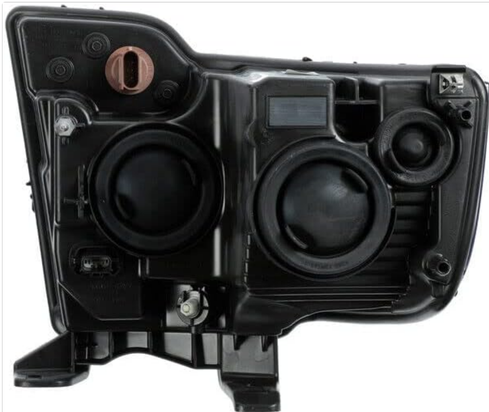
Image 2.2: Rear view of the headlamp assembly, highlighting the access points for bulbs and electrical connections, crucial for installation and maintenance.
