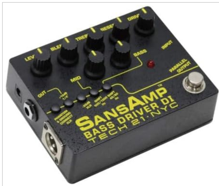
Figure 3: Side view showing XLR and 1/4" outputs.
