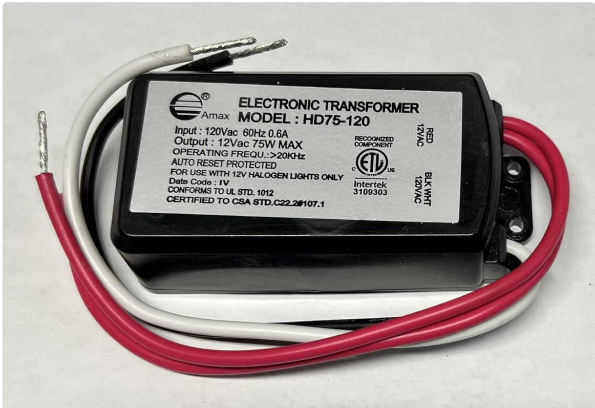
Figure 1: Import HD75-120 Electronic Low Voltage Halogen Transformer. The label displays input (120Vac 60Hz 0.6A) and output (12Vac 75W Max) specifications, operating frequency (>20KHz), auto reset protection, and certification details (cETLus Intertek 3109303, UL STD. 1012, CSA STD.C22.2#107.1). Wiring includes black/white for 120VAC input and red/white for 12VAC output.
