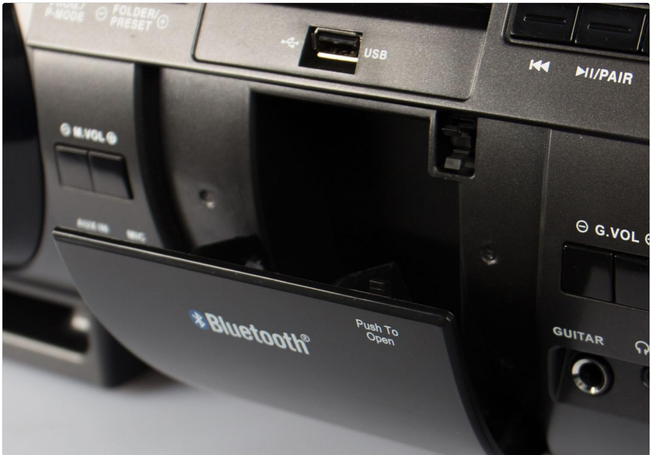
Figure 4.2: Close-up of the Blaupunkt BB 1000's USB port and Bluetooth indicator, located within a protective compartment.
