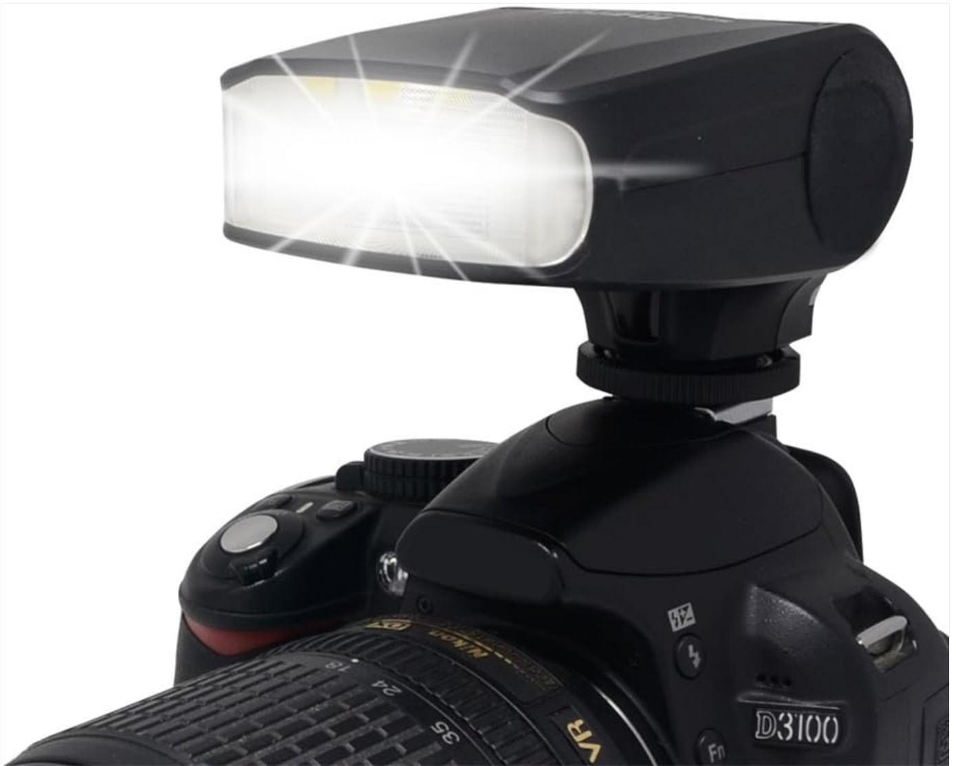
Figure 4: Hot Shoe Connection. The metal hot shoe base and locking ring ensure a secure connection.
