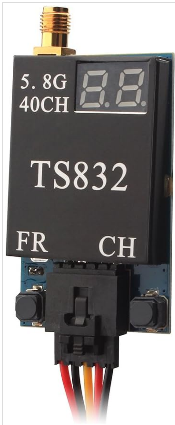
Figure 5: The TS832 Transmitter showing its wiring harness for connecting to an FPV camera and power source.
