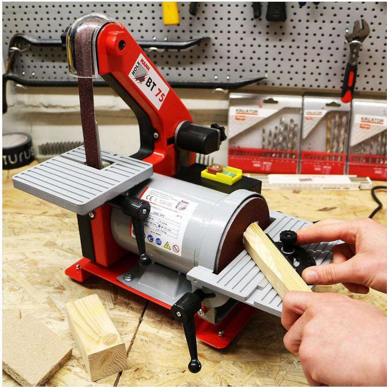
Figure 7: A user demonstrating the use of the disc sander to smooth a wooden block, utilizing the adjustable work table.
