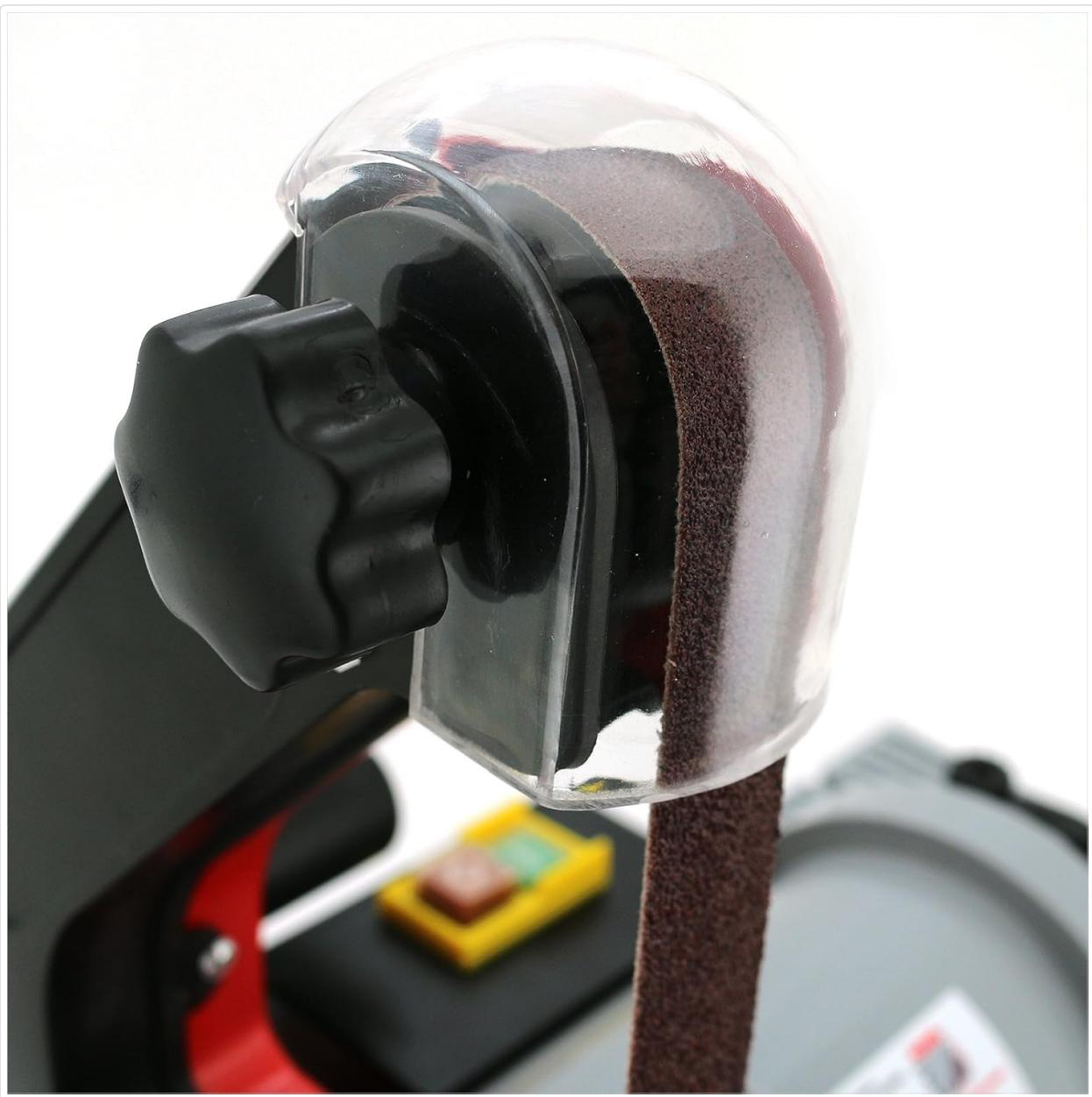
**Figure 3:** Close-up view of the transparent guard covering the sanding belt, ensuring user safety during operation.
