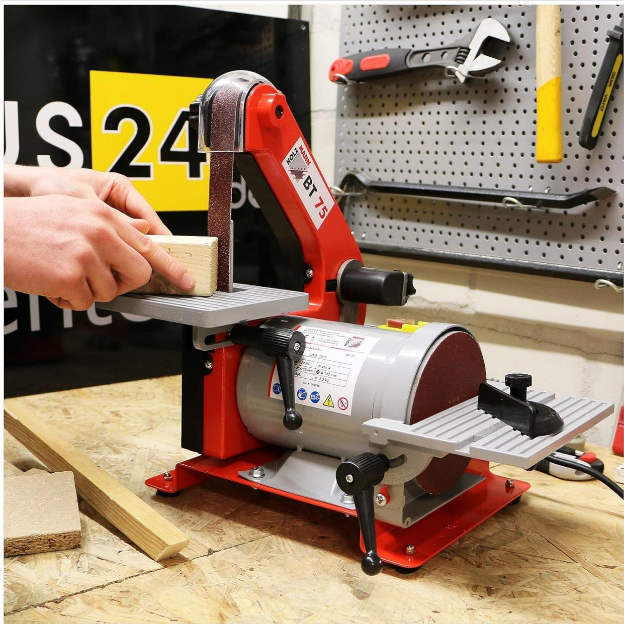
Figure 6: A user demonstrating the use of the band sander to smooth the edge of a wooden block.
