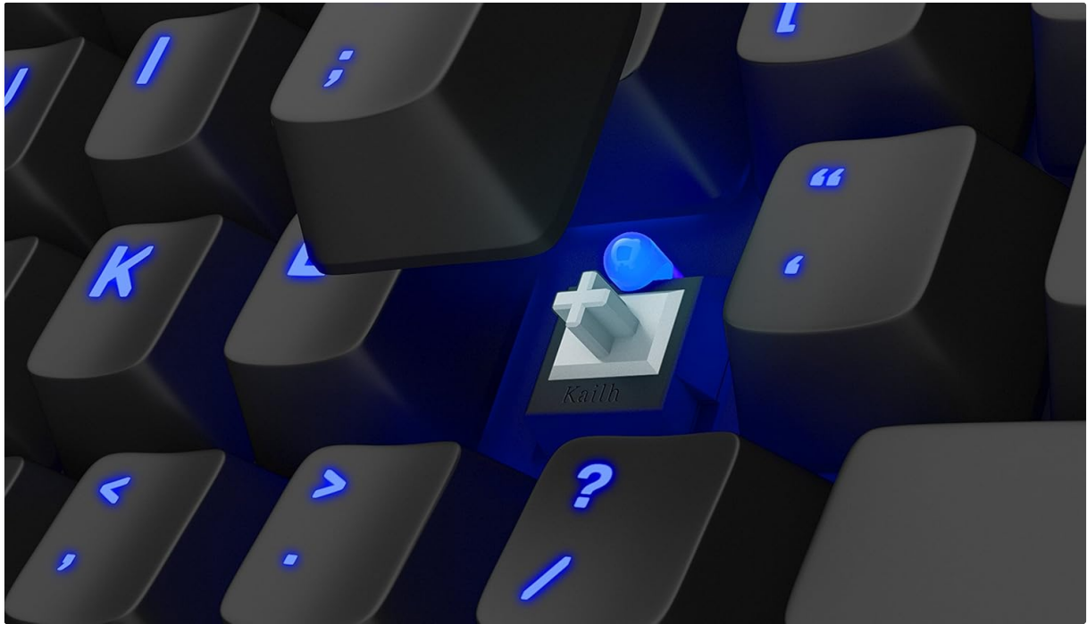
Figure 4: A close-up of a keycap, showing the Kailh mechanical switch and the blue LED illumination beneath it.
