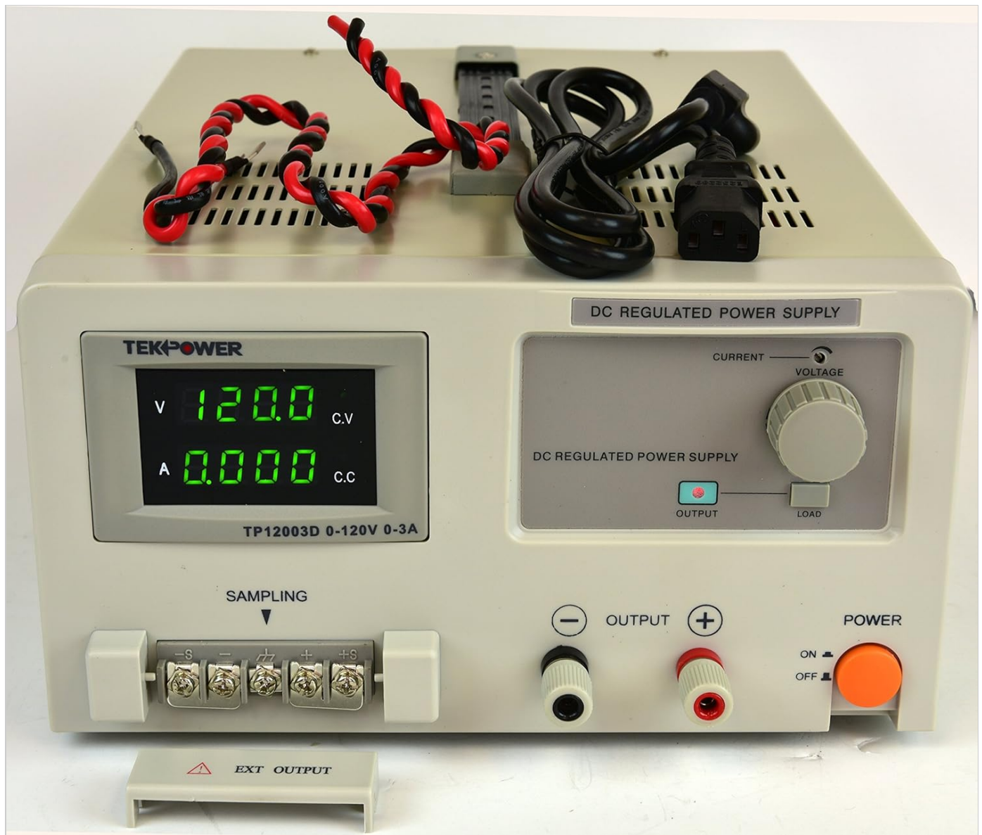
Figure 3.1: Tekpower TP12003D unit with power cord and alligator clip probes.
