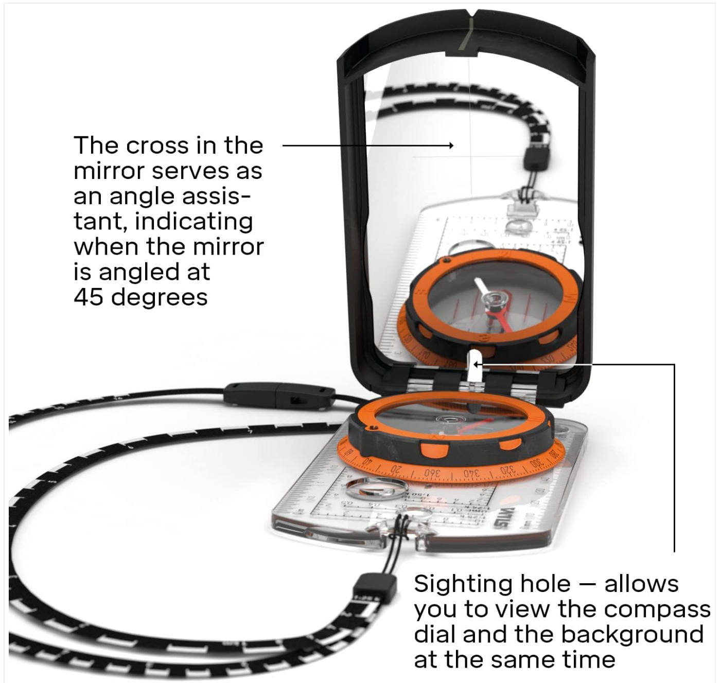
Image: The mirror of the compass, illustrating how the cross serves as an angle assistant for 45-degree angles, and the sighting hole for simultaneous viewing of the dial and background.
