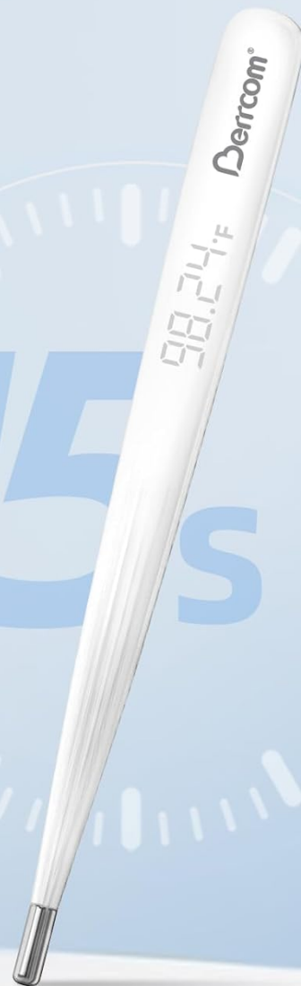
Image 3.1: Easy to Use Features. This graphic highlights the thermometer's high accuracy ( \pm 0.01^{\circ}\text{F} ), storage charging, IPX65 waterproof rating, auto-off function, vibration alert, and last memory record.
