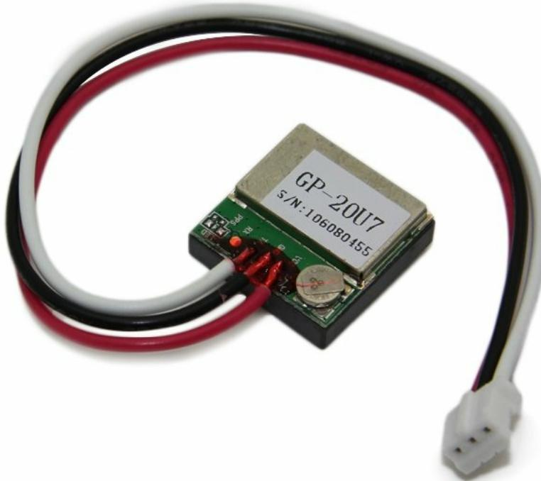
Figure 1: Sparkfun SF-GPS-13740 Sensor GPS IC GP-20U7 module. This image shows the compact GPS module with its integrated GP-20U7 chip, connected to three wires (red, black, white) ending in a white connector. The module itself is green with a silver component labeled "GP-20U7 S/N: 106080455".
