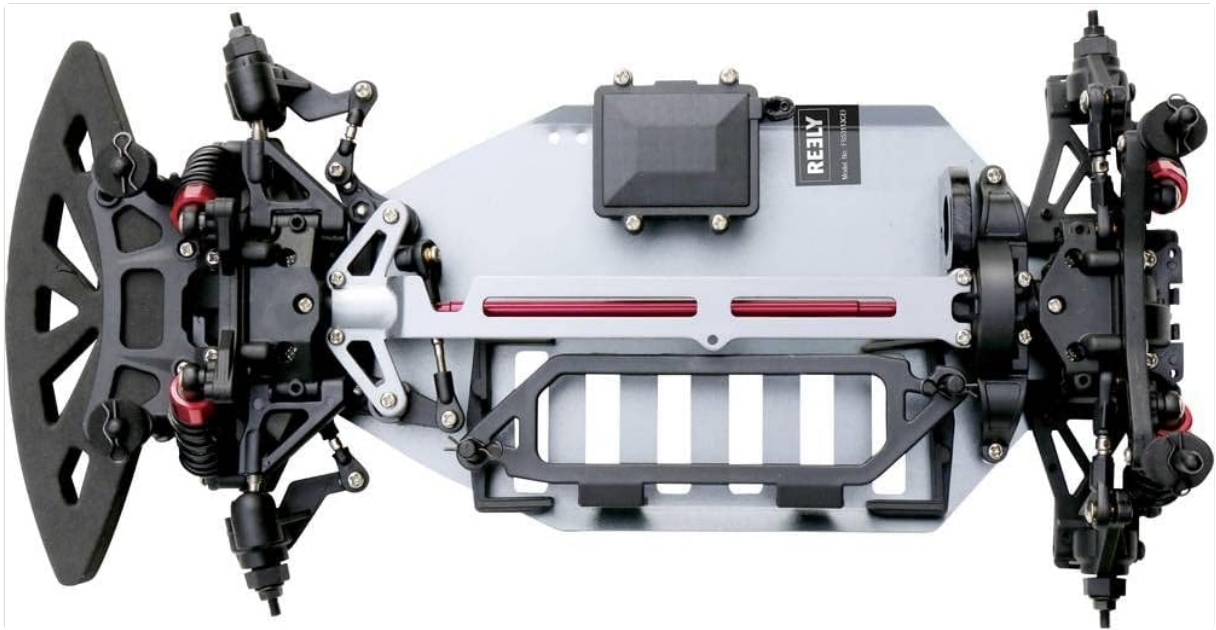
Image: Top-down view of the REELY FS53113CEI chassis. This perspective clearly shows the central layout of the chassis, the 4-wheel drive system, and the mounting points for electronic components.
