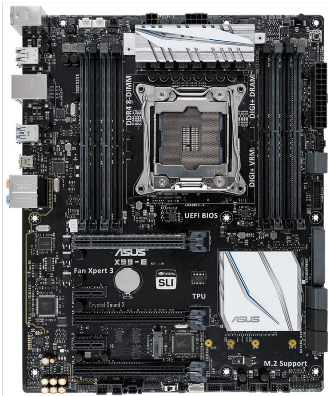
Figure 1: ASUS X99-E LGA2011-v3 ATX Motherboard. An overhead view showcasing its LGA2011-3 CPU socket, eight DDR4 DIMM slots, PCIe slots, M.2 support, and various connectors. Key features like Fan Xpert 3, Crystal Sound 3, and the ASUS Aura RGB header are visible.
