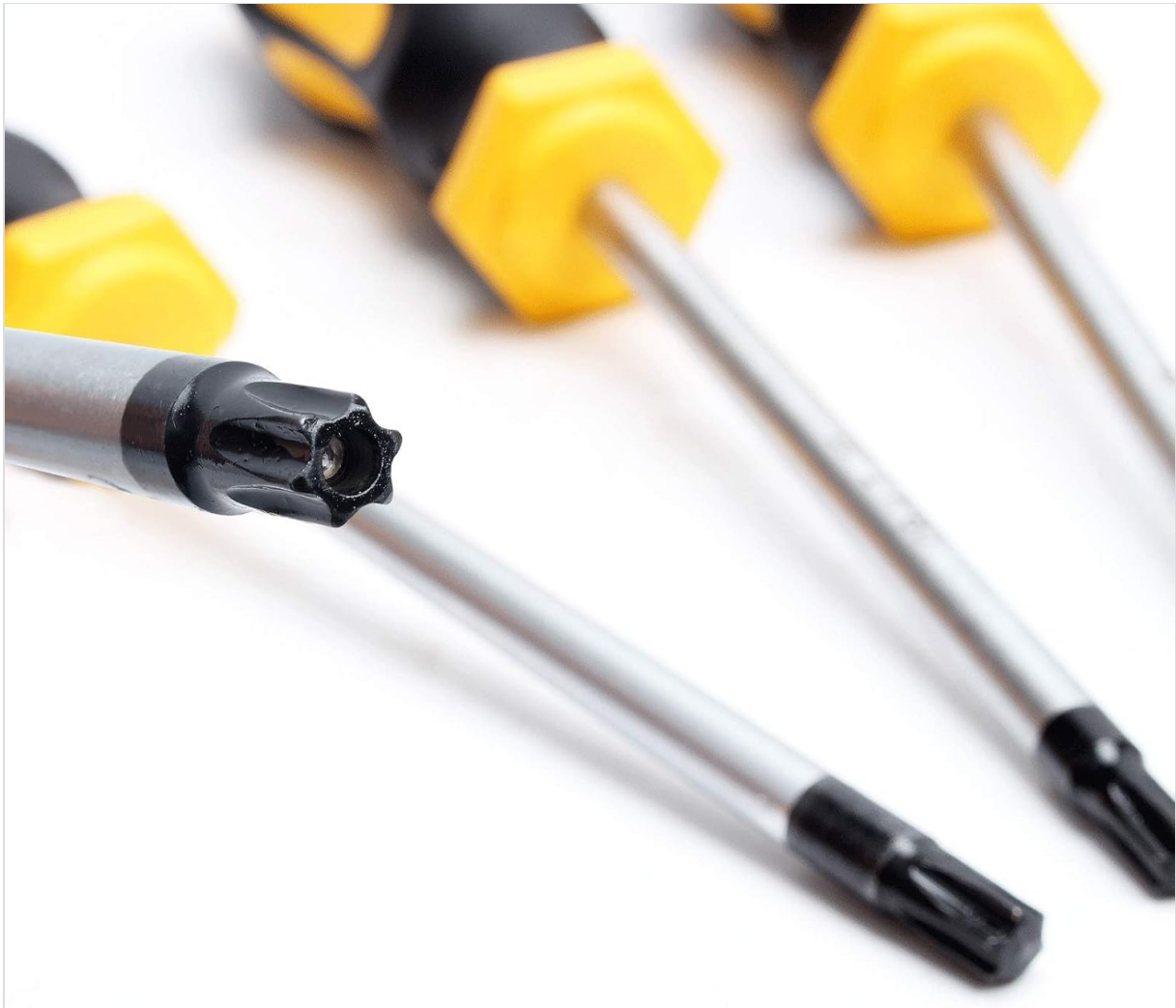
Image 3.1: Detail of a Torx screwdriver tip with a security hole.
