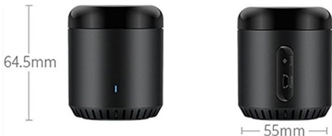
Figure 2: Dimensions of the Broadlink RM Mini3 (64.5mm height, 55mm width).
