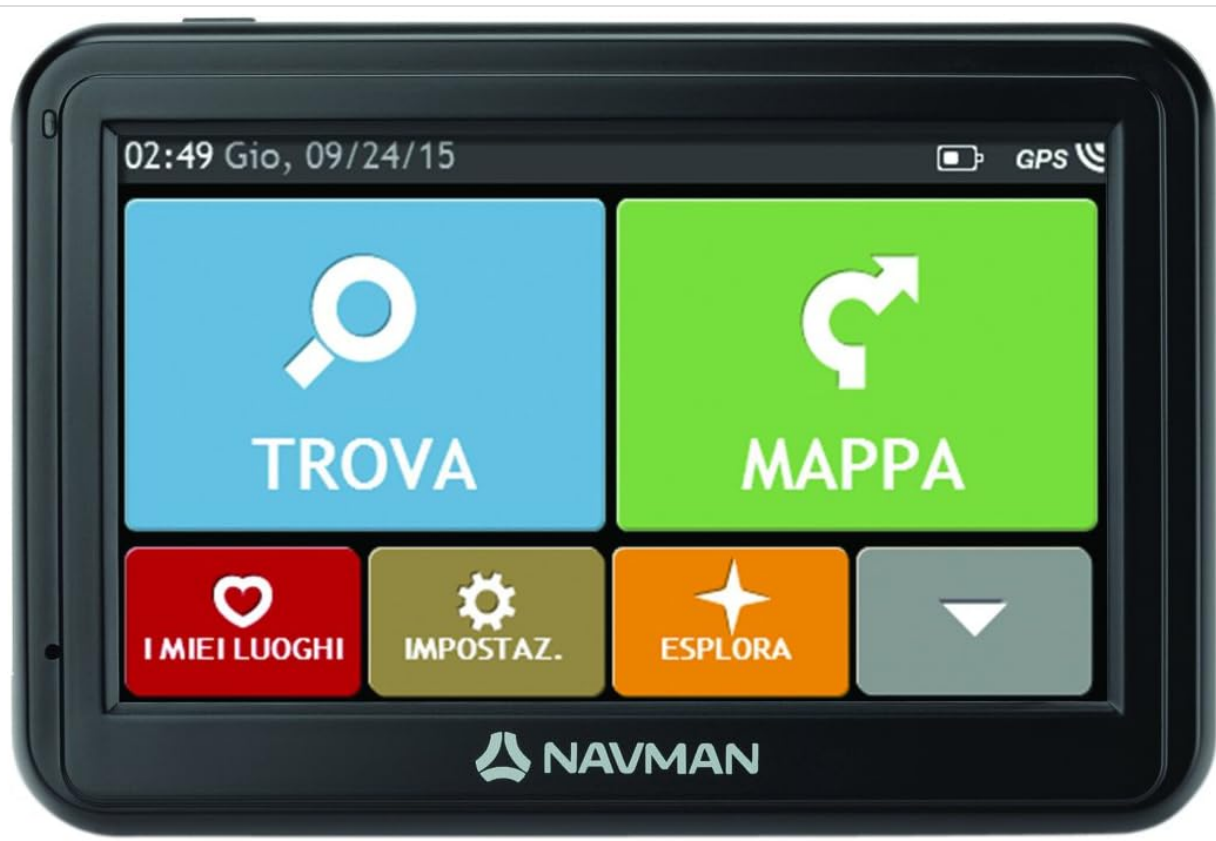
Figure 1: This image shows the Mio Navman 4000 GPS device powered on, displaying its primary user interface. The screen features large, touch-friendly buttons for key functions such as 'TROVA' (Search), 'MAPPA' (Map), 'I MIEI LUOGHI' (My Places), 'IMPOSTAZ.' (Settings), and 'ESPLORA' (Explore). The top bar indicates the current time, date, battery status, and GPS signal strength. This is the typical screen you will see upon starting the device.
