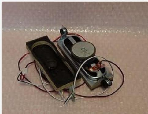
Image: RCA LED55G55R120Q Speakers. This image displays two speaker units, one with a rectangular black enclosure and the other featuring a circular silver component, both connected by various wires, indicating their internal nature for integration into a larger system.
