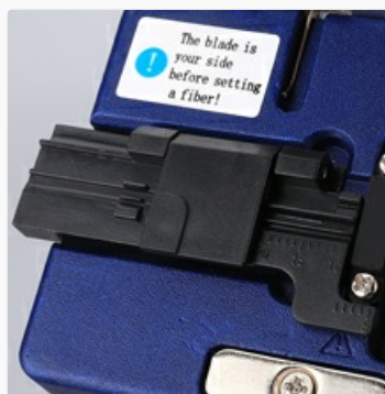
Figure 4.1: Proper placement of the fiber in the cleaver's fixture.
