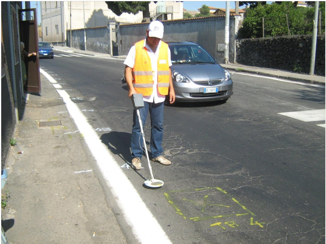
Figure 4.1: An operator demonstrating the proper sweeping technique with the CS880 metal detector on an asphalt surface.
