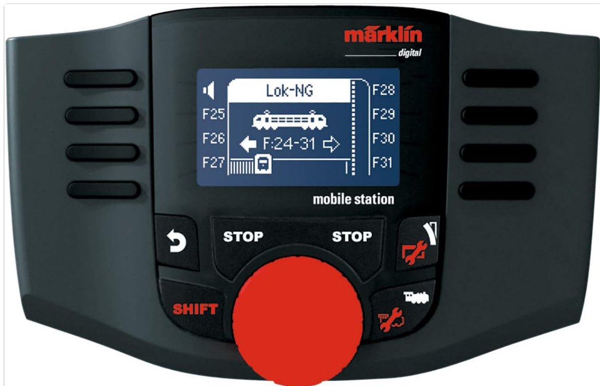
Figure 2: The Mobile Station display showing active locomotive functions (F24-F31) and a locomotive icon.
