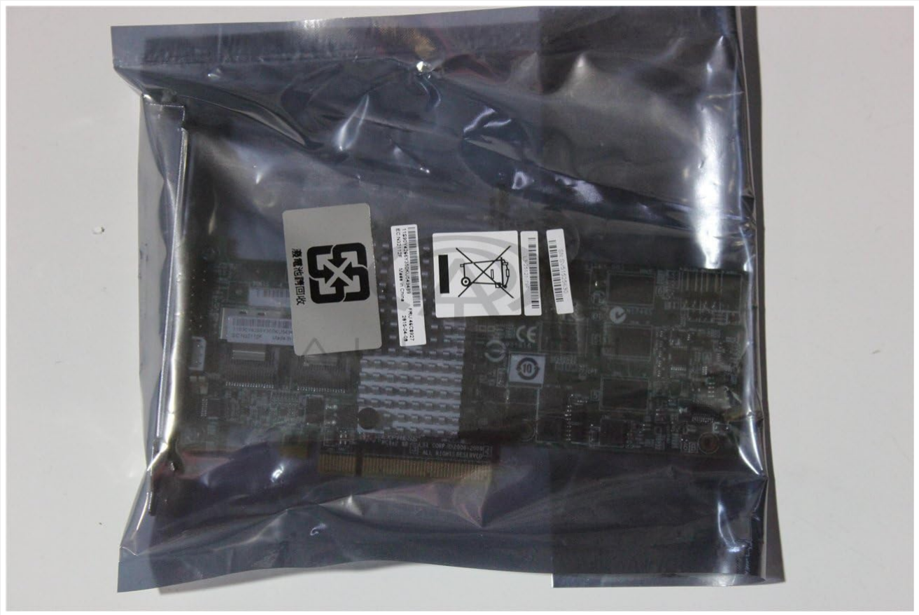
Figure 3: The IBM ServeRAID M5015 controller packaged in an anti-static bag, emphasizing the importance of ESD protection during handling.
