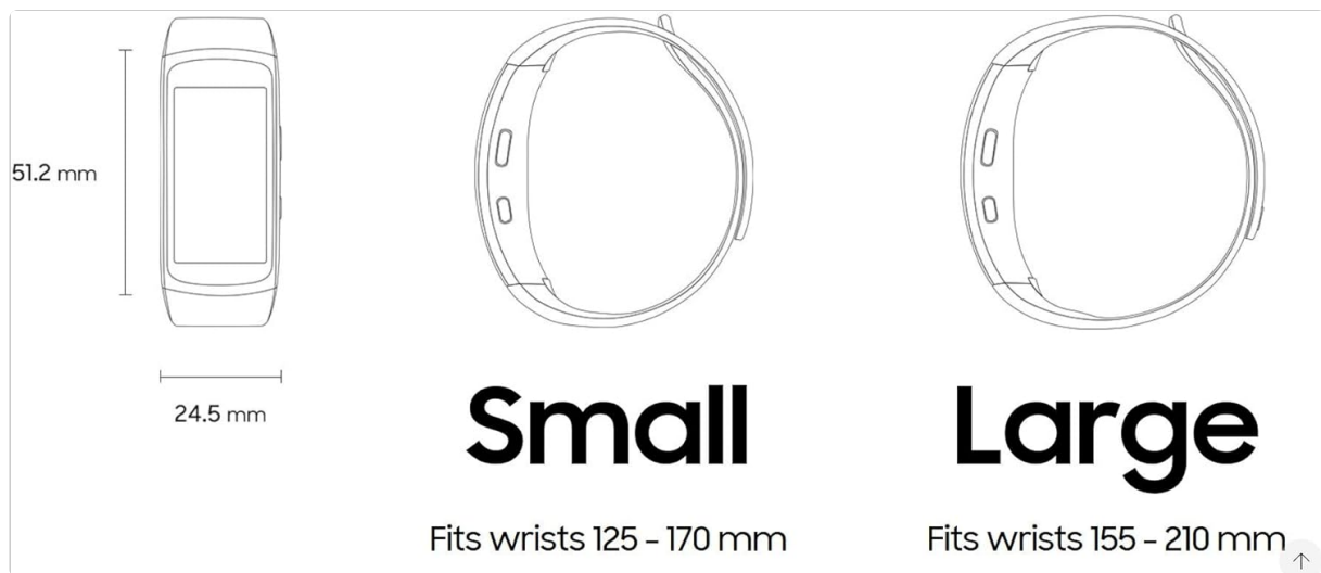
Figure 2: Illustration showing the dimensions of the Gear Fit2 and the size differences between the small (125mm-170mm) and large (155mm-210mm) band straps.
