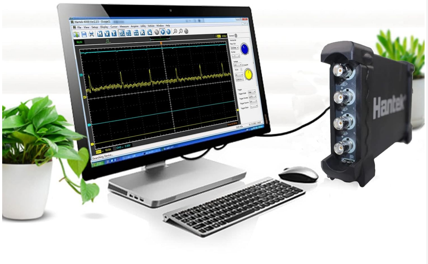
Figure 5.1: The Hantek 6074BE oscilloscope connected to a desktop computer, demonstrating a typical setup for operation.
