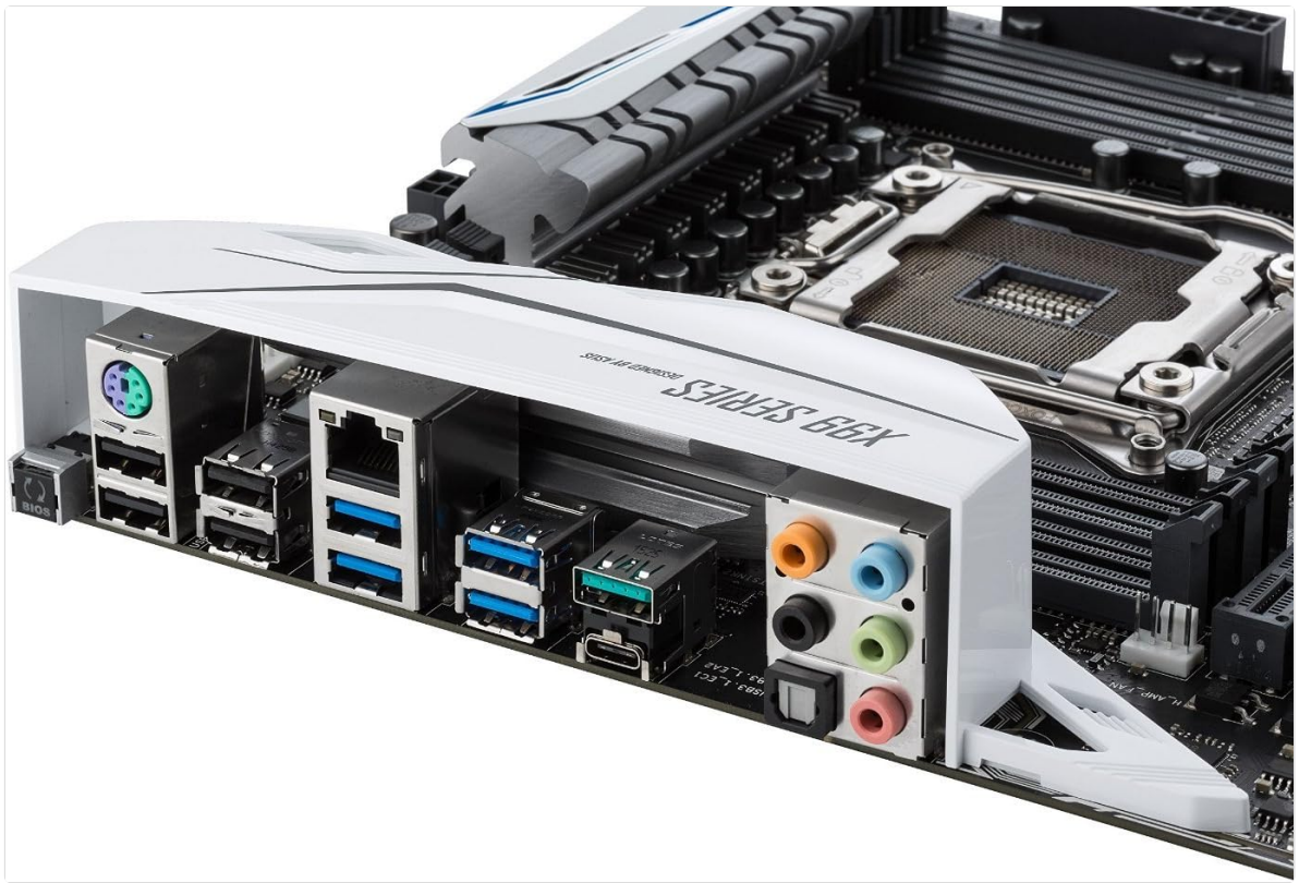
Image: Close-up view of the rear input/output (I/O) panel of the ASUS X99-A II motherboard, showing USB ports, Ethernet, audio jacks, and other connectors.
