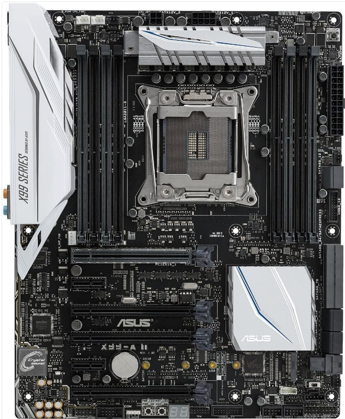
Image: Top-down view of the ASUS X99-A II motherboard, illustrating the CPU socket, DIMM slots, PCIe slots, and various headers.
