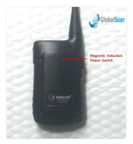
This image shows the location of the magnetic induction power switch on the remote transmitter.
