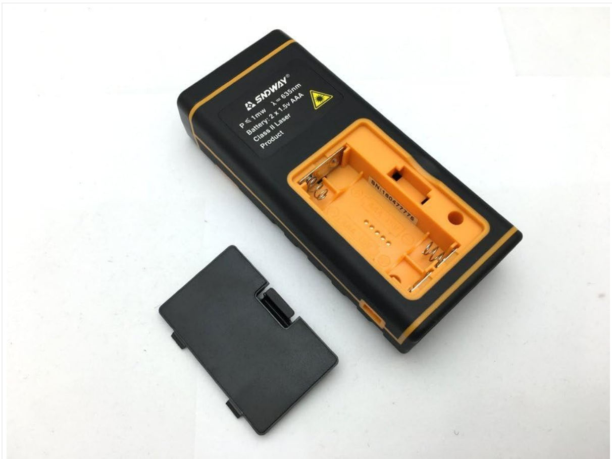
Figure 5: Rear view of the SNDWAY SW-T80 with the battery compartment open, showing where to insert two AAA batteries.
