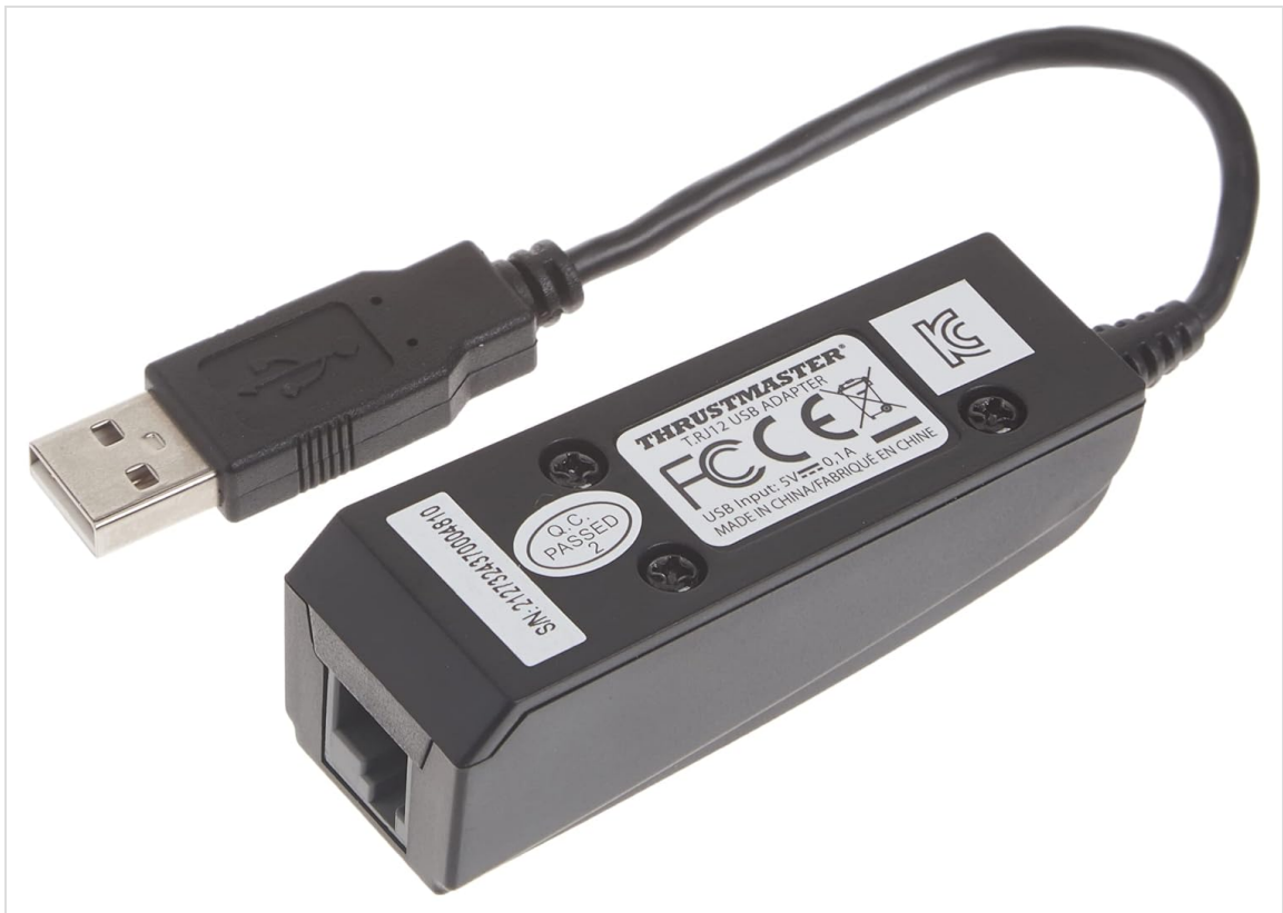
Image: The underside of the adapter, displaying its model information and regulatory compliance.
