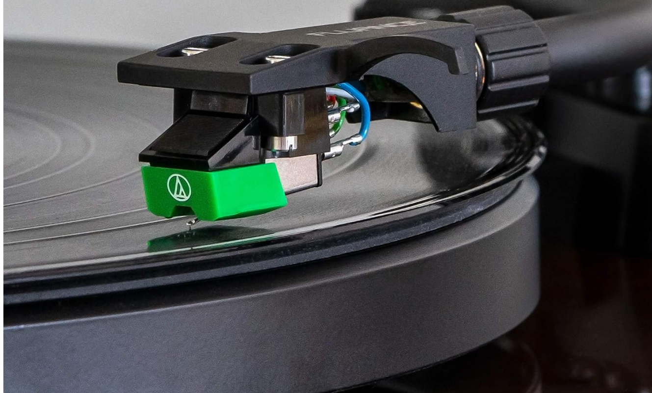
Image: A close-up view of the Fluanice RT81 turntable's tonearm, highlighting the Audio Technica AT95E cartridge with its green stylus.
