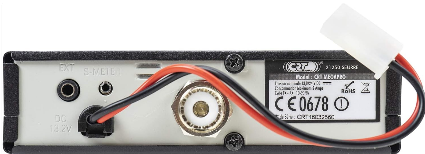
Image: Rear view of the CRT MegaPro CB radio, showing the antenna connector, power input, and external speaker/S-meter jacks.
