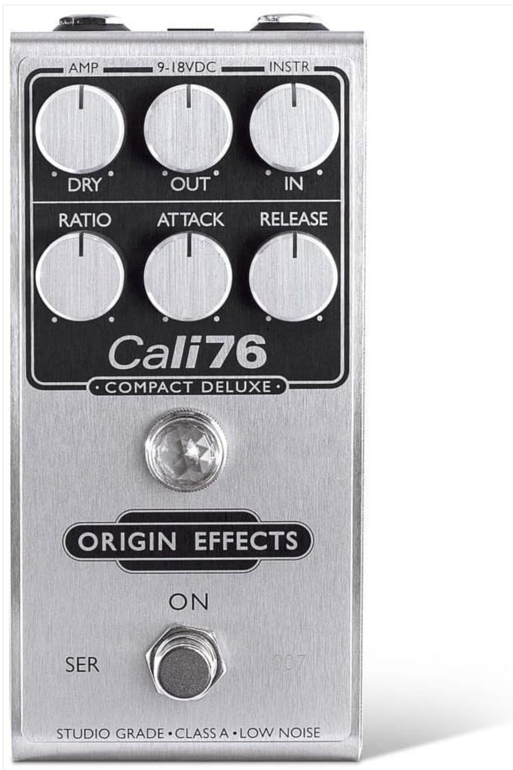
Figure 1: Front view of the Cali76 Compact Deluxe pedal, highlighting the control layout.
