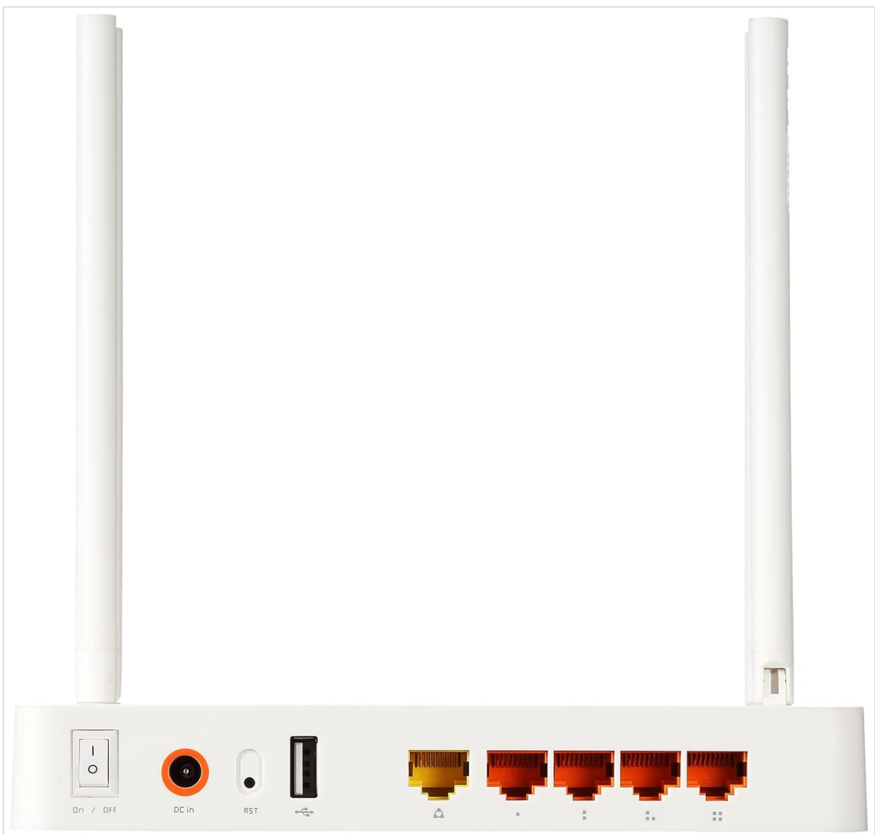
Figure 3.2: Rear panel of the TOTOLINK A3002RU-V2 router, displaying the power switch, DC input, Reset button, USB 2.0 port, WAN port, and four LAN ports.
