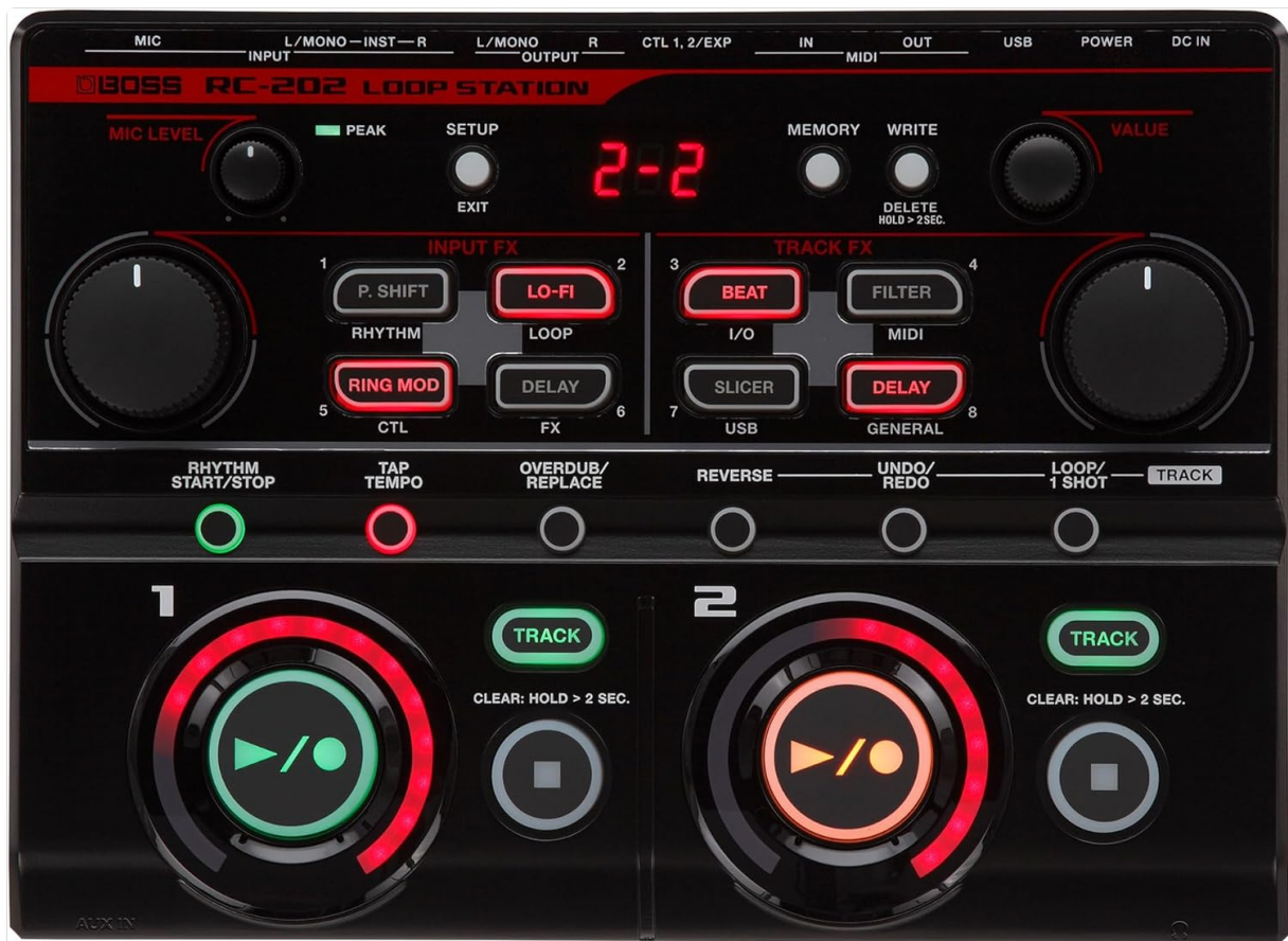
Image: The main control panel of the RC-202, featuring two distinct loop tracks with play/record buttons, stop buttons, and track-specific controls.
