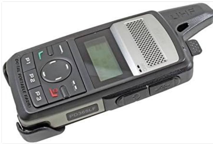
Figure 1: Hytera PD365LF Digital Portable Radio. This image displays the radio from an angled perspective, highlighting its compact form factor. Visible features include the speaker grille, LCD screen, navigation buttons (P1, P2, P3, and a central directional pad), and the UHF antenna. The model number "PD365LF" is clearly visible on the front casing.
