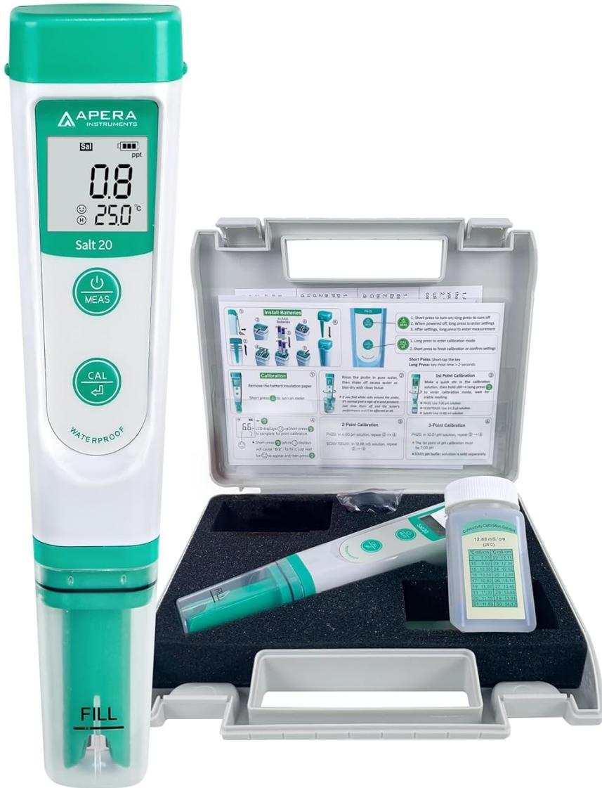
The Salt20 Salinity Tester Kit includes the meter, calibration solution, AAA batteries, and a lanyard, all housed in a portable carrying case.
